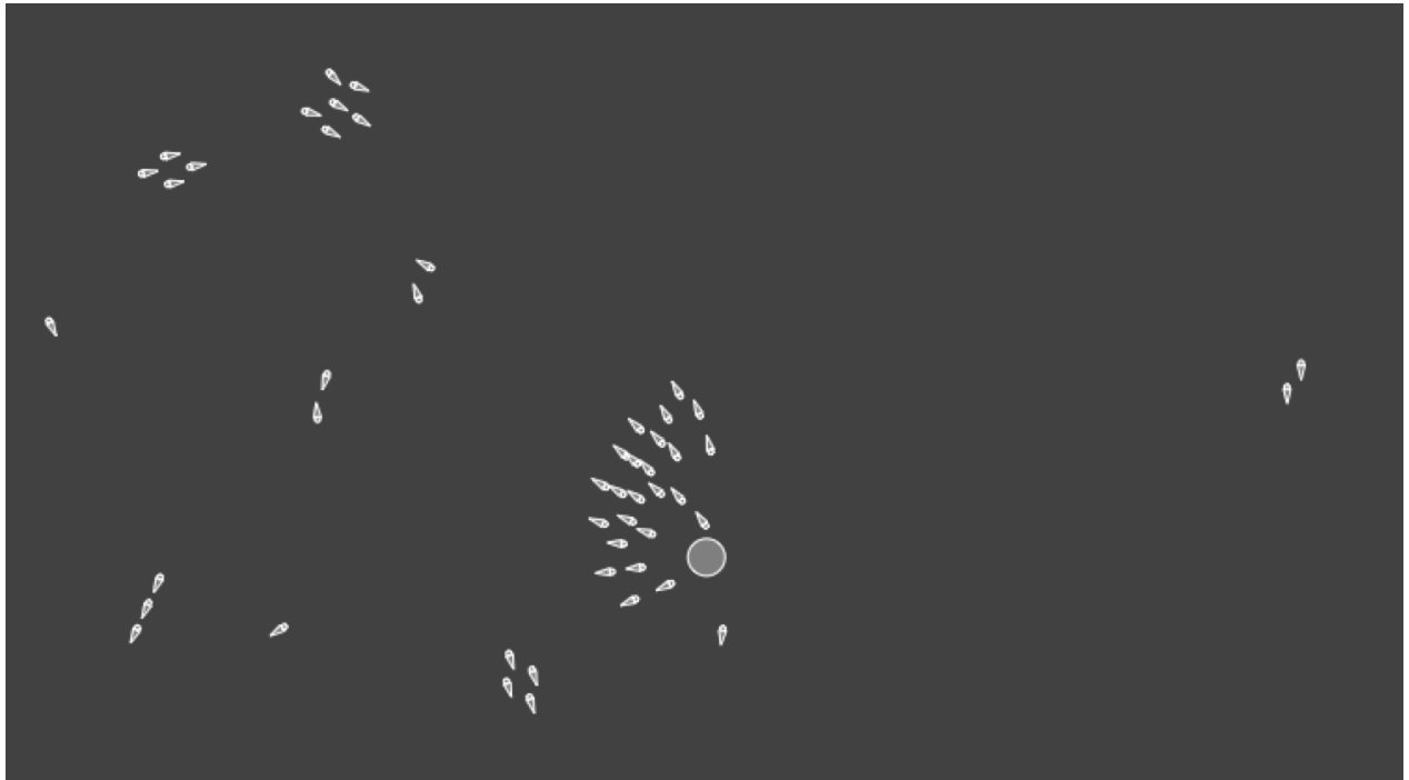
Flocking test in processing, implementing modified Reynolds algorithm
