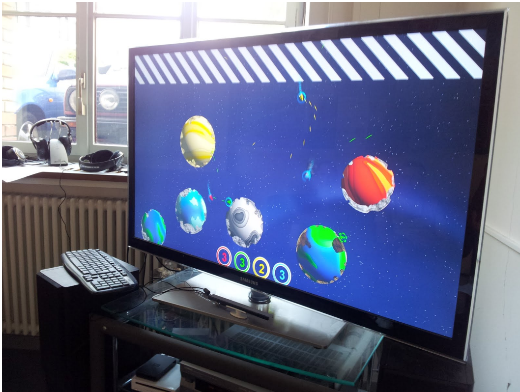
Fig 5.2: The huge plasma TV we used for playtesting. Bottom shows some issues with safe-zoning, and colors are more intense than on computer screens.
