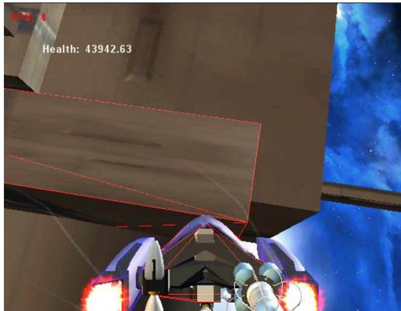
Figure 8: Red: Convex hulls that collide; Blue: Convex hulls that are taken into account for collision from the sphere based collision search tree
